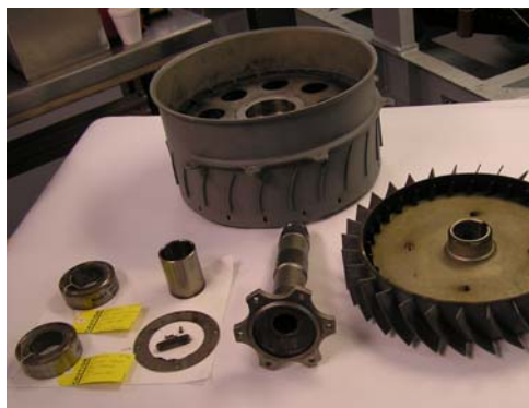
Fig. 2: H-60 oil cooler components.
