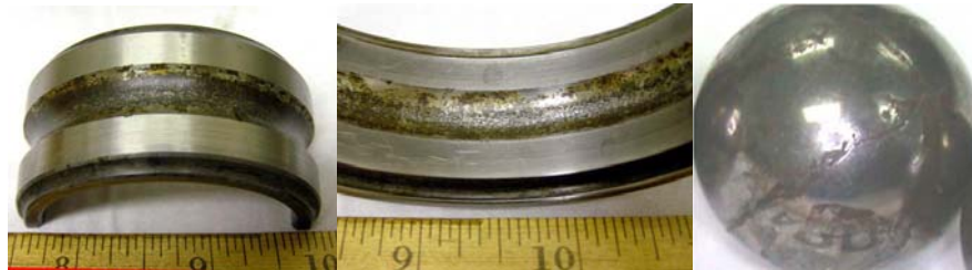
Fig. 3: Oil cooler bearing degradation: corroded inner raceway (left) and outer raceway (middle), and damaged bearing ball (right).
